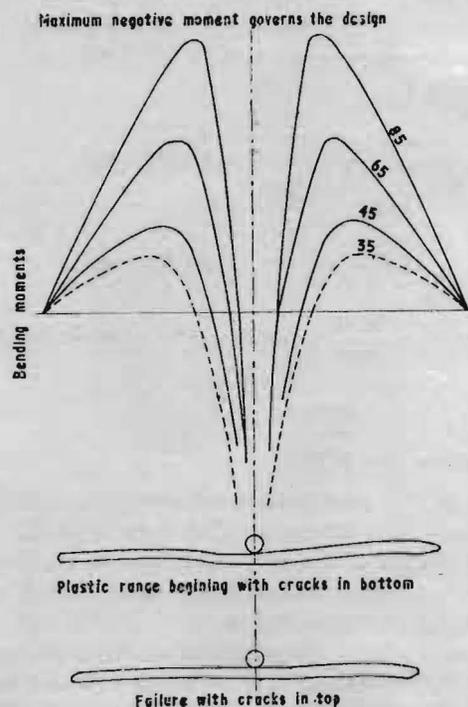
Fig 2 Bending in plastic range
