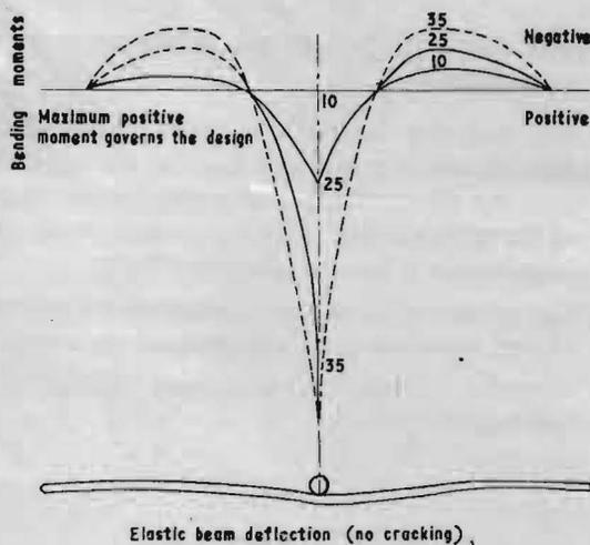
Fig 1 Bending in elastic range
