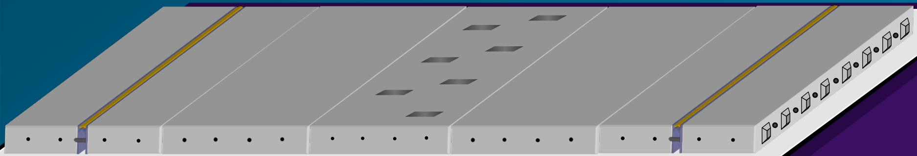
**Joint Panel   Base Panel   C.S. Panel   Base Panel   Joint Panel**
